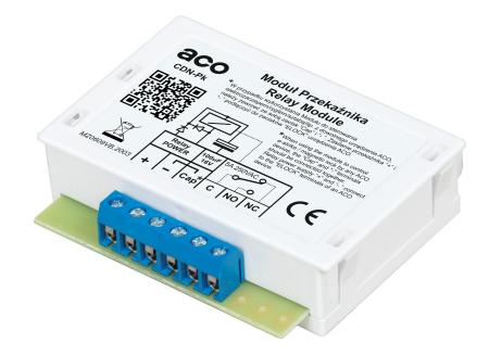
Universal relay module with easy connection via screw terminals. It enables, among other things, the connection of a traditional electric door strike, electromagnetic lock, door controller, reversing door strike or any other device. It has a built-in capacitor, which allows the module to work with ACO devices that have an output to connect only the electric door strike.
